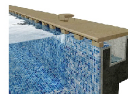
No 11 Overflow Systems
